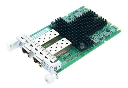
LRES3029PF-OCP is a dual-port 25G Ethernet network adapter with OCP3.0 SFF structure developed by Shenzhen Lianrui Electronics Co., LTD based on Intel E810 chip. Virtualization applications with 1/10/25G connection to meet network infrastructure, based on the RDMA feature of iWARP, RoCEv2 to achieve direct memory to memory data communication between applications over the network.
